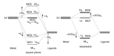
A simplified MO treatment shows that the amount by which each MO is shifted in energy on forming the complex can be expressed in terms of a single energy parameter  $e_{\sigma}$ . For example, MO1 is shifted down in energy by  $3e_{\sigma}$ , whereas MO8 is shifted up in energy by  $\frac{4}{3}e_{\sigma}$ . MO3 and MO7 are nonbonding and so do not change energy.
