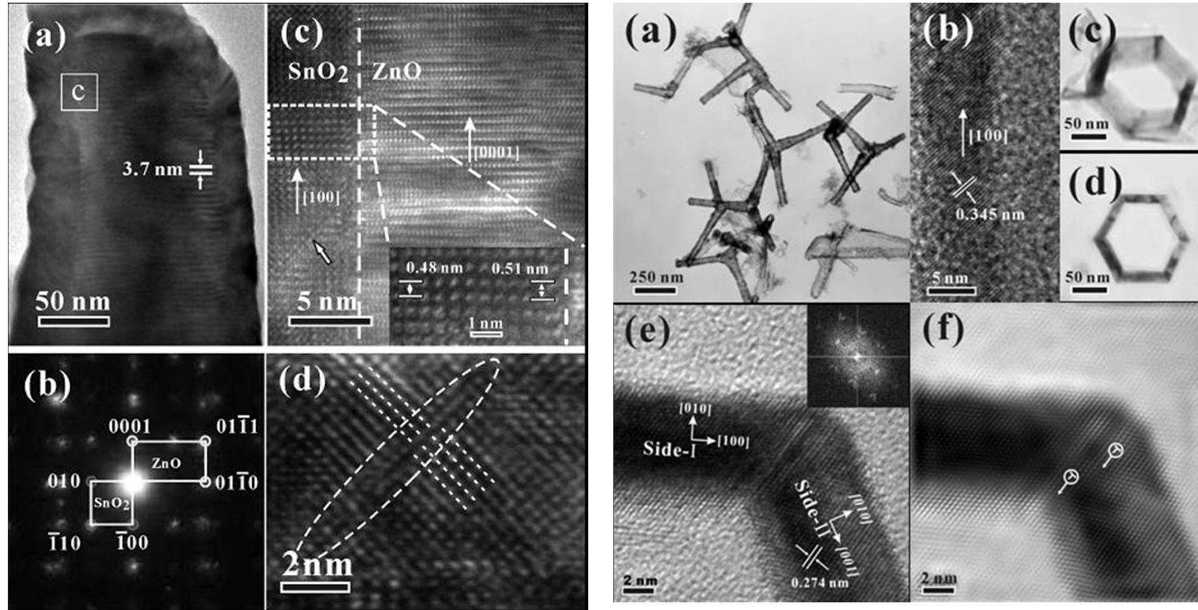
Epitaxial relationship :  $(010)_{\text{SnO}_2} \parallel (0110)_{\text{ZnO}}$  and  $[100]_{\text{SnO}_2} \parallel [0001]_{\text{ZnO}}$
