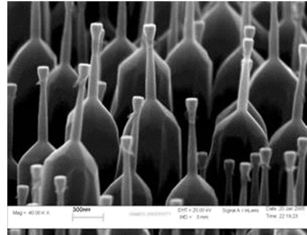
Micro-wave plasma CVD of ZnO on Silicon surfaces
