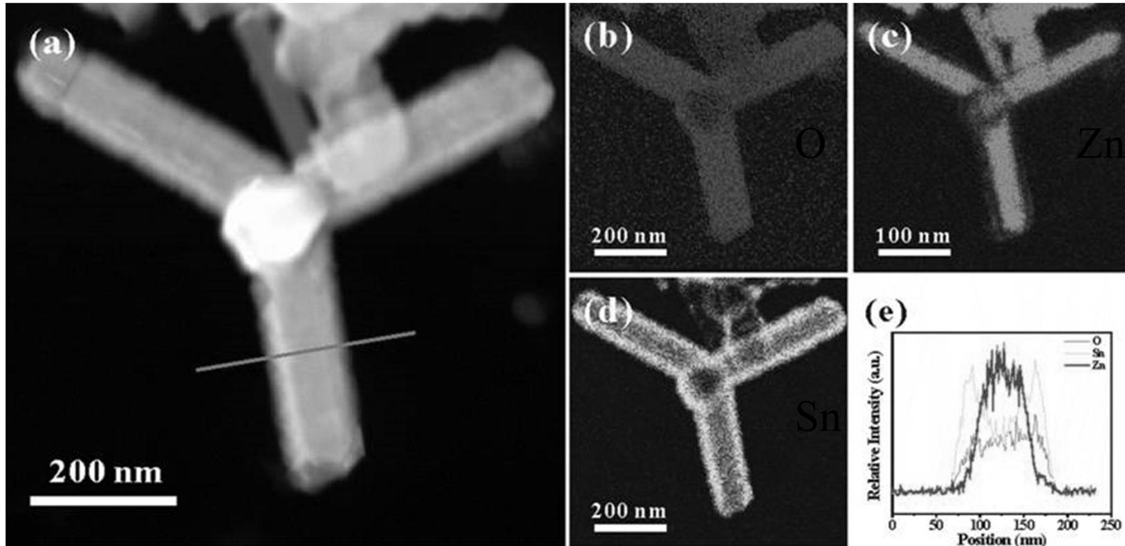
**(SnH<sub>4</sub> flow rate = 10 sccm, deposition time = 5 min)**
