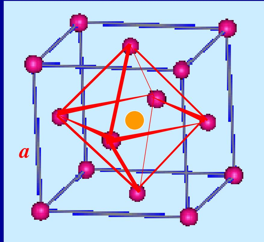
For a close-packed structure formed from identical spheres of radius  $R$ , the octahedral hole size is  $0.414R$ .
