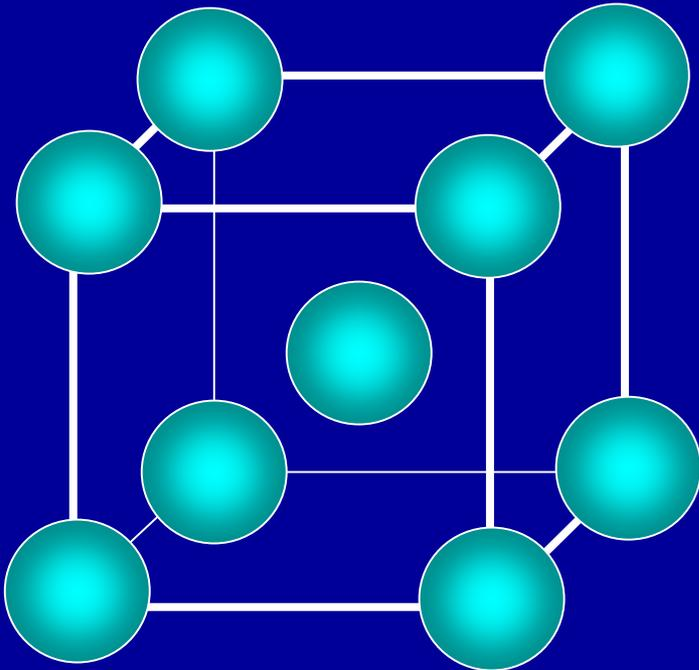
Each unit cell has two spheres(atoms).
