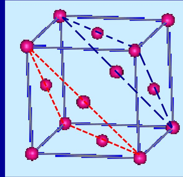
The volume of the unit cell :  $V_{cell} = a^3 = (4R / \sqrt{2})^3 = 16\sqrt{2}R^3$
