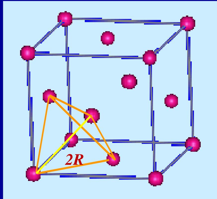
For a close-packed structure formed from  $N$  spheres of radius  $R$ , the tetrahedral hole size is  **$0.225R$** .
