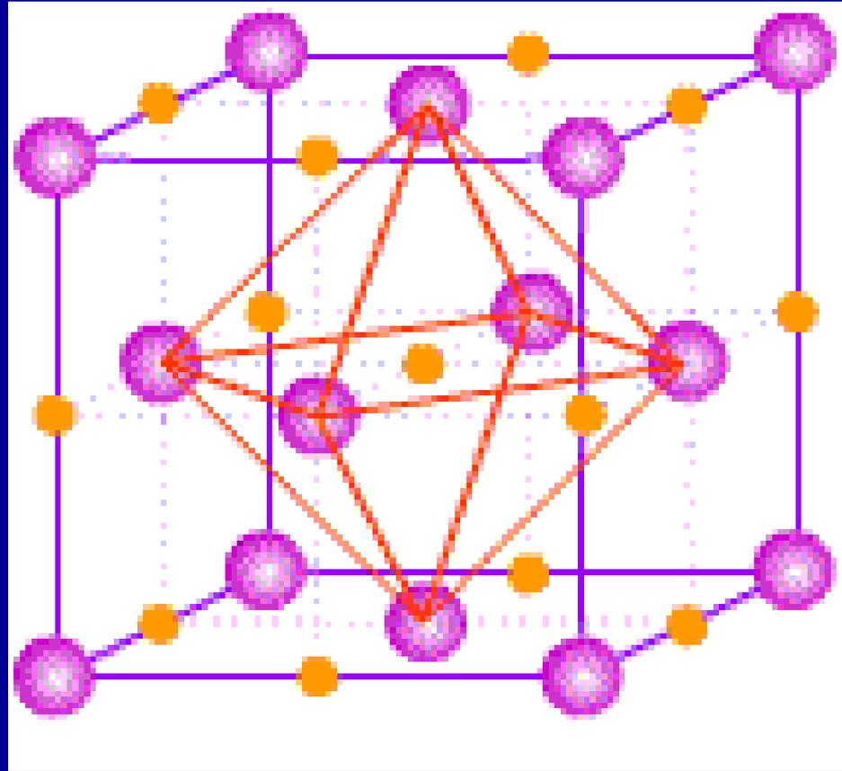
b. **Ferrite**(铁素体): a solid solution of C in  $\alpha$ -Fe. Since the size of the octahedral holes is very small in  $\alpha$ -Fe, the solubility is very low (the highest solubility is 0.02%)
