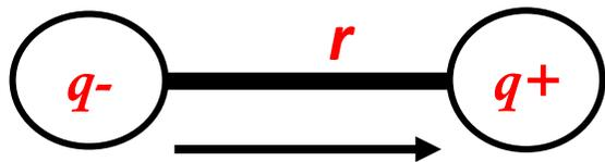
$$\vec{\mu} = \vec{r}q = 4.8 \times \vec{r}(\text{\AA}) \times q(e) \text{ D}$$
